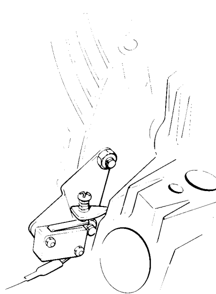
Fig. H10. By-Pass Micro-Switch
