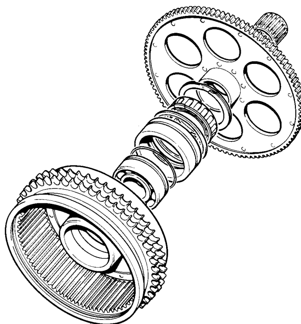
Fig. C7 Starter Gear and Freewheel Bearing
