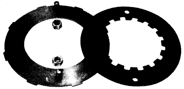
FIG. 24 Tool to Stop Engine Turning
