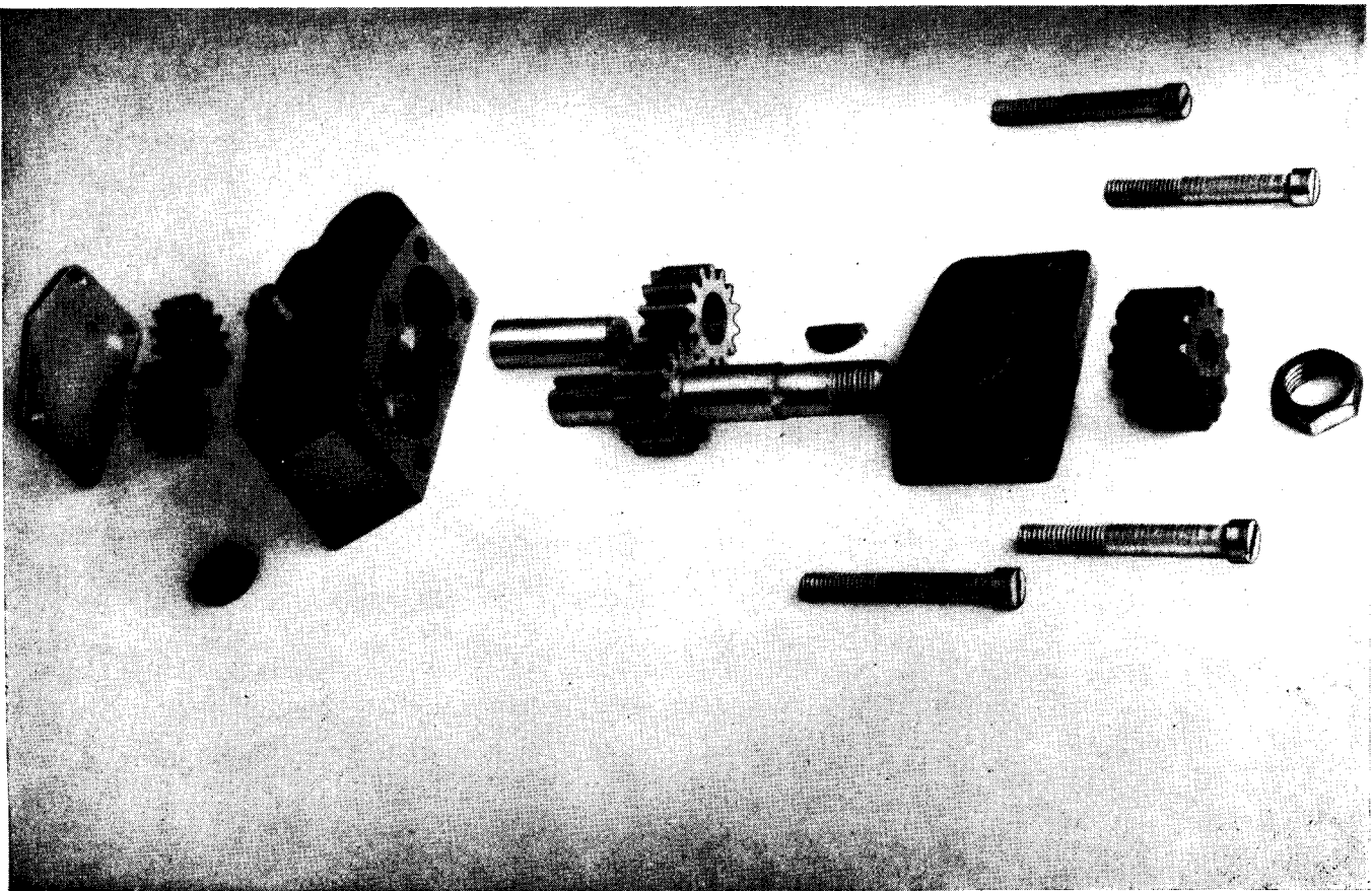
FIG. 1 The Oil Pump
