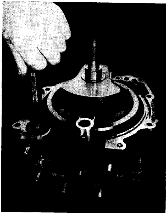
FIG. 16 Extracting the Camshaft
