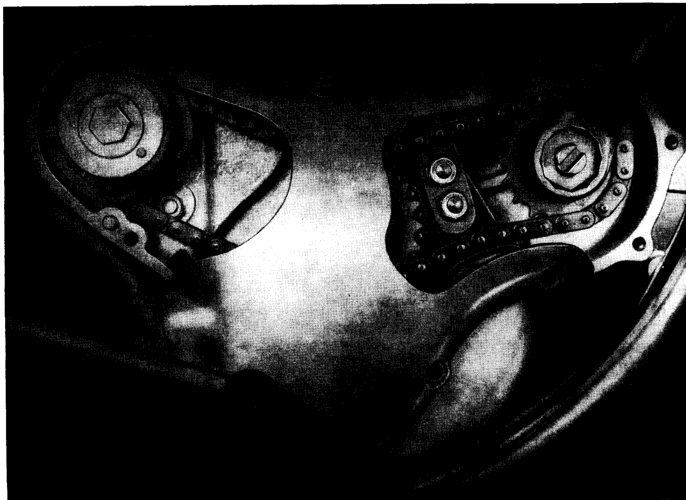
FIG. 15 Cut-Away Timing Cover
